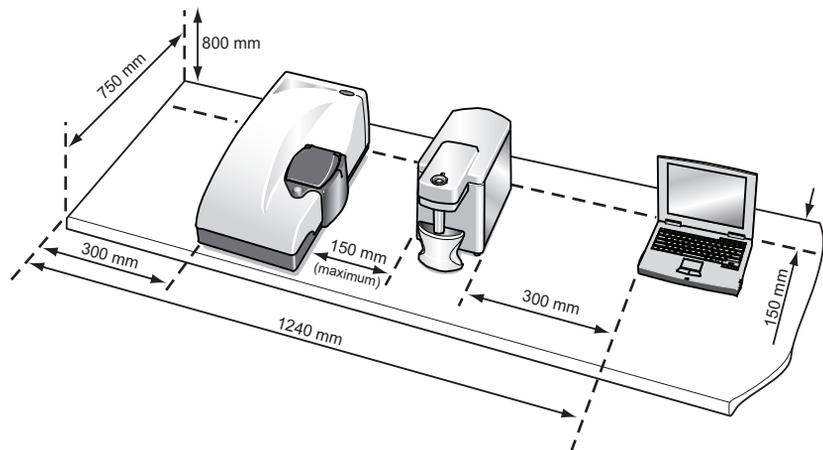
Allow at least **800mm** above the bench surface for access to the cell area. The system dimensions are given below (the width is with the cuvette holder closed):
