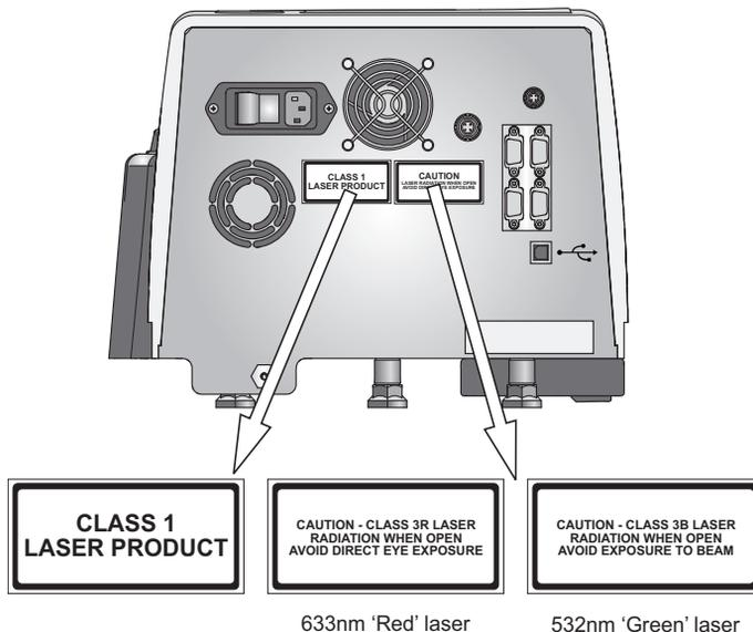
The standard laser has a maximum cw-power of 4mW at 632.8nm, while the option laser has a maximum cw-power of 50.0mW at 532nm.
